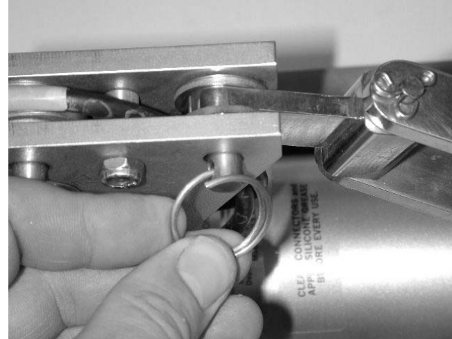
STEP 1. SECURE MAG. TOWCABLE TERMINATION TO SSS TOWFISH BY INSERTING THE CLEVIS PIN (P/N 16200050) THROUGH THE TOWBRACKETS, FLAT WASHERS (ITEM 5), AND .25 IN THICK (6MM) CONNECTION TAB. INSTALL COTTER RING (P/N 16200044) AS SHOWN.
