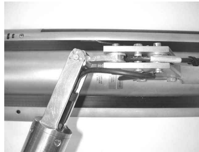
STEP 4. CHECK RANGE OF MAG. TOWCABLE TERMINATION MOTION. CABLES SHOULD NOT BIND OR PINCH. ADJUST CABLE LENGTHS AND POSITION AS NECESSARY.
