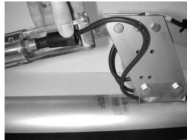
STEP 2. CLEAN AND APPLY LIGHT A COATING OF SILICONE GREASE TO THE CONNECTOR PINS (IF NEEDED) AND MATE CONNECTORS. TIGHTEN LOCKING SLEEVE AS SHOWN.
