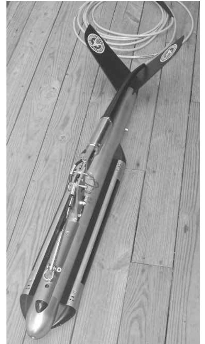
SSS TOWFISH AND MAGNETOMETER TOWCABLE INSTALLED.
